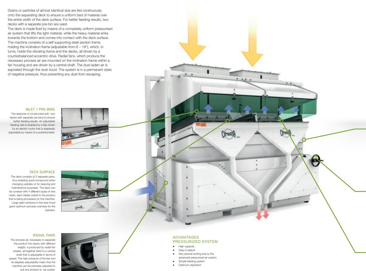
CONSTRUCTION AND PRINCIPLES BASED ON PROVEN TECHNOLOGY
